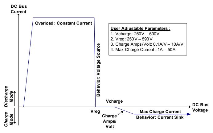
The V-I (Voltage and Inductance) curve (see **Figure 44**) shows the performance characteristics and modes of operation of the Liebert FS system based on the seven user-configurable system parameters.
